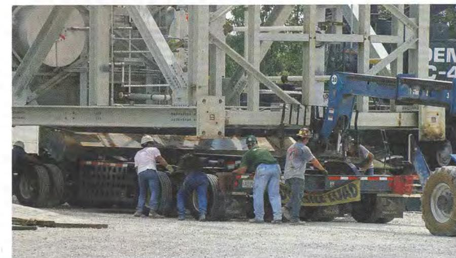
A Trail King steerable dolly was used to haul the largest module. The convoy required three escorts, two bucket trucks for powerlines and a service truck
