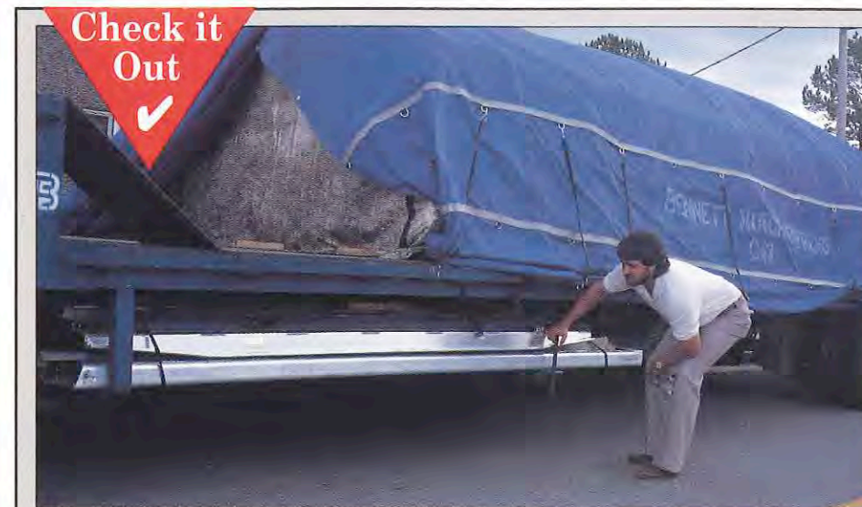
David Lowry checks stowed ramps, which add cargo versatility to Bennett's dropdeck trailers.
